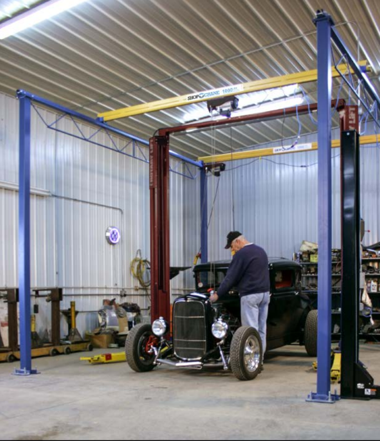
This 12' x 12' system features a second bridge to easily handle longer objects.
