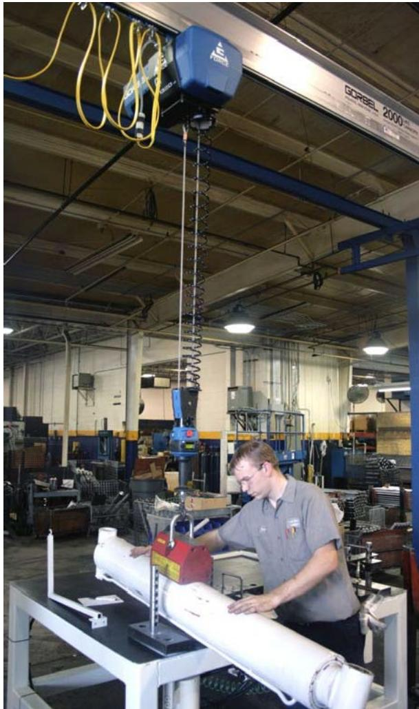
The company had several chain hoists throughout the facility, but wanted a lifting device that gave operators more control and maneuverability when handling the large cylinders. When Nomax Solutions brought in a G-Force® for a demonstration with the company's work force, they found that the best solution was right in their hands.
