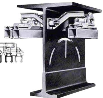
Steel brackets, which mount directly on the track web, support conductors on 10" and larger patented track. These supports can be turned up or down, depending on track depth and wheel size. One to six conductors can be held by the off-web supports.
